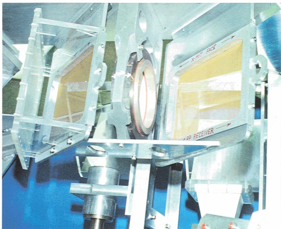
FIGURE 12. The completed quasi-optical circulator in the BWG system. The Faraday rotator is at a beam waist, and each of the two polarization filters is mounted at an angle of 45° to the beam path. A membrane supported by a plexiglass holder at the left is a -40-dB quasi-optical coupler that functions as the peak-power monitor for the system.
