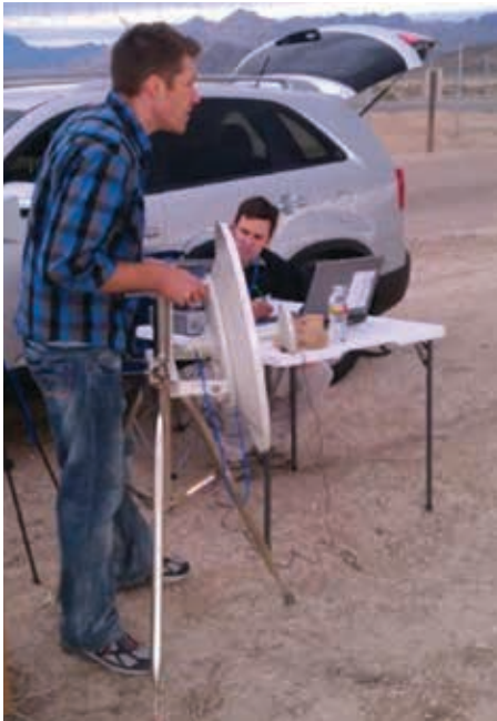
LEFT: Lincoln Laboratory researchers Matt Johnson and Ben Bullough collect RF signals from a tactical system during field tests that were used to assess potential cyber vulnerabilities of the system.
