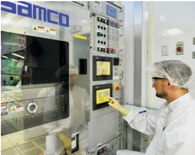
William Spencer is working at the SAMCO oxide deposition system in the compound-semiconductor fabrication room. This system is used to deposit oxide films as part of the many device fabrication steps required for the demonstration of record performance slab-coupled optical waveguide lasers (SCOWs) and amplifiers (SCOWAs).
