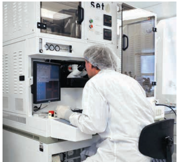
Al Ruff is operating a flip-chip bonding tool that is used to align and attach Geiger-mode avalanche photodiodes (APD) to readout integrated circuits (ROIC). An example of a dual 128 x 32 APD/ROIC integrated module is shown left.
