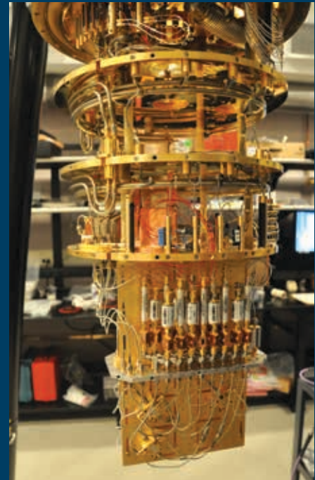
Dilution refrigerator for experiments on superconducting qubits.
