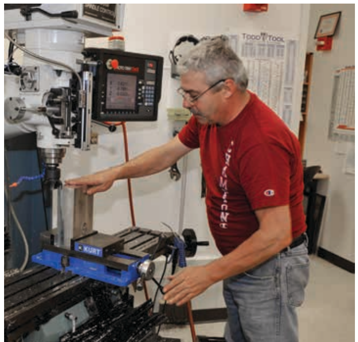
Machinist Russell Gouveia sets up new billet of aluminum to be machined into a complex part for an aircraft pod program.
