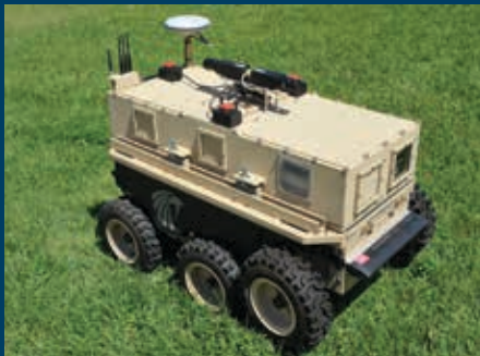
The Outdoor Unmanned Ground Vehicle Navigation program is developing algorithms and infrastructure to enable robust unmanned navigation of both structured and unstructured (e.g., woodland) environments. In 2011, the Patrol Leader platform (above), autonomously traversed a prerecorded course (right) at Moore Army Airfield while maintaining a constant standoff distance in front of a human-occupied vehicle.
