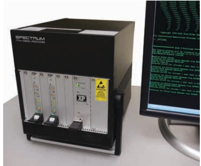
The next-generation, airborne collision avoidance system, ACAS X, initial hardware prototype is currently undergoing bench testing.
