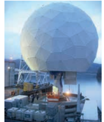
Lincoln Laboratory completed the mechanical installation of all components of the X-band Transportable Radar (XTR-1), the large-scale, ship-based RF system. Shown clockwise from far left are the reflector installation, feed installation, the radome being lowered over the dish, and the completed radar on the Pacific Tracker .
