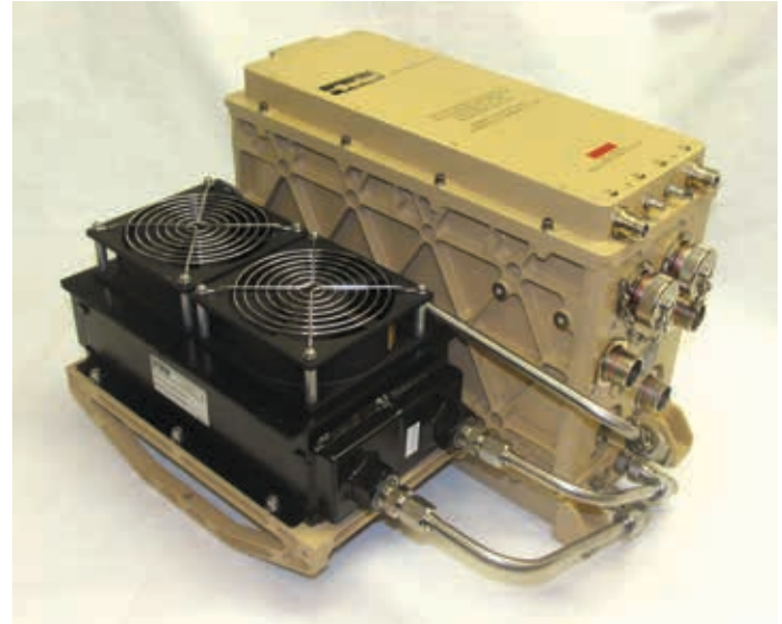
ABOVE AND RIGHT: The Laboratory is developing a novel ground-penetrating radar capability to be used by combat engineers. An initial prototype has been integrated onto an Army Husky vehicle.
