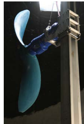
Submersible Mixer on Support Pole
