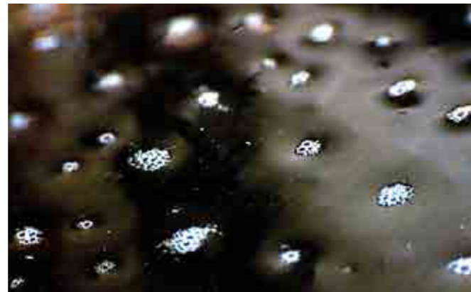
Presence of macro foam in wet clear coat
