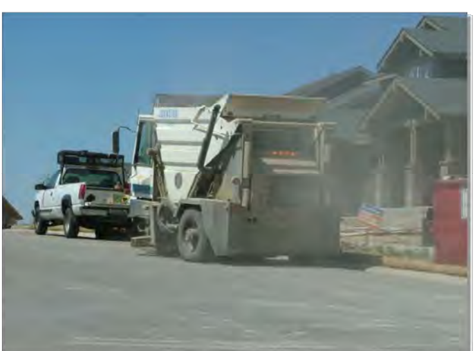
Photograph SS-1. A street sweeper removes sediment and potential pollutants along the curb line at a construction site.
