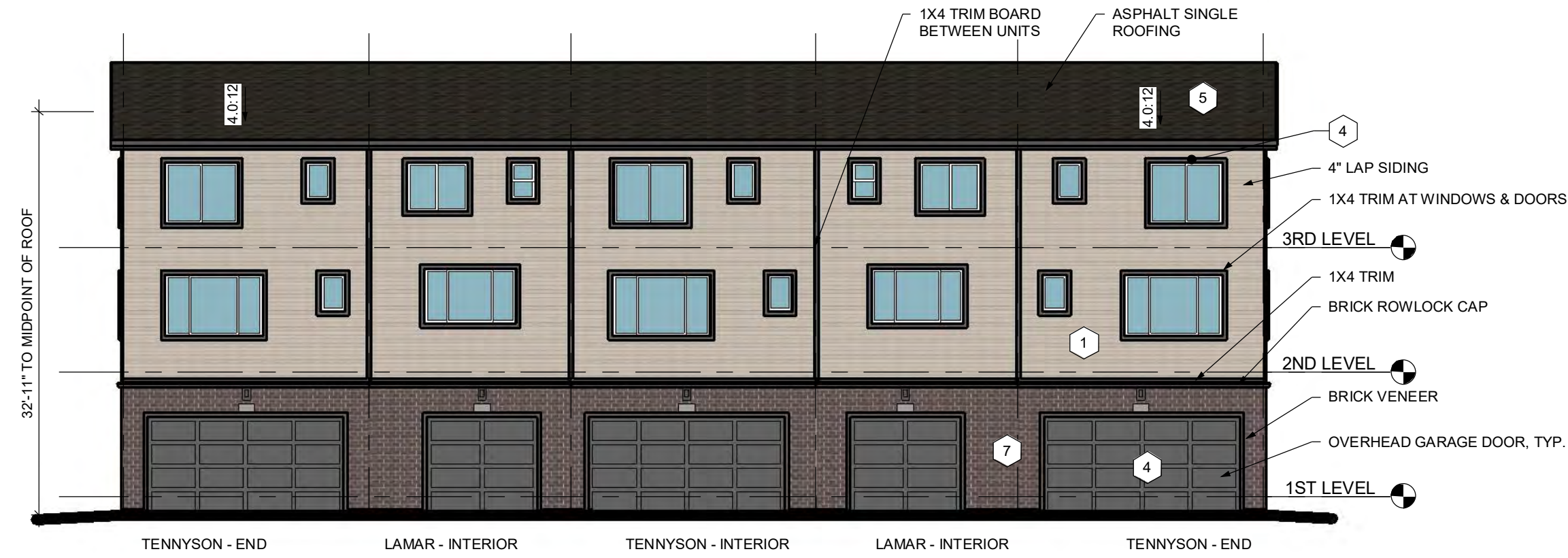
4 3-STORY REAR LOAD - 5-PLEX-B - REAR ELEVATION 3/32" = 1'-0"
