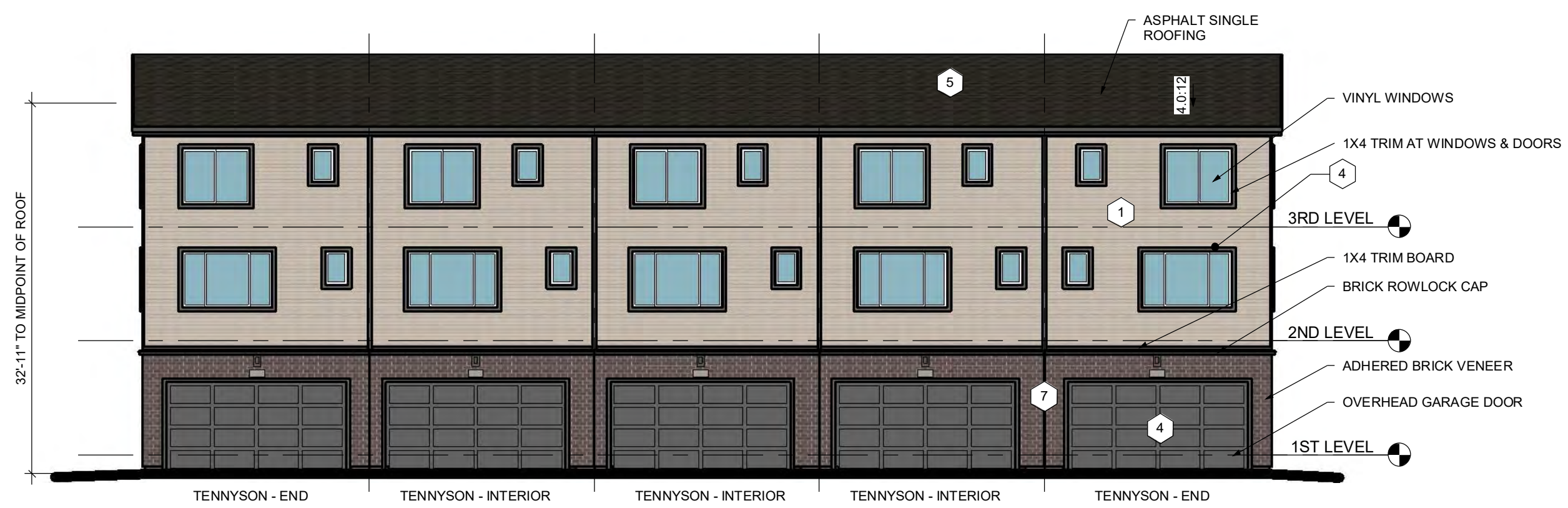
4 3-STORY REAR LOAD - 5-PLEX - REAR ELEVATION 3/32" = 1'-0"
