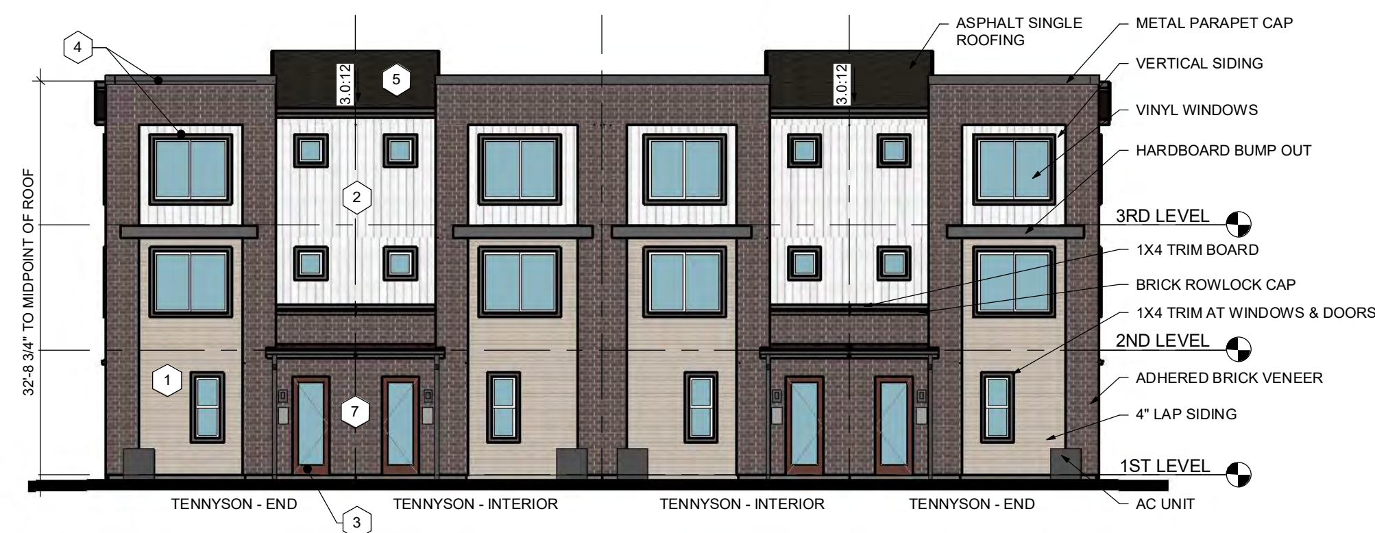
1 3-STORY REAR LOAD - 4-PLEX - FRONT ELEVATION 3/32" = 1'-0"
