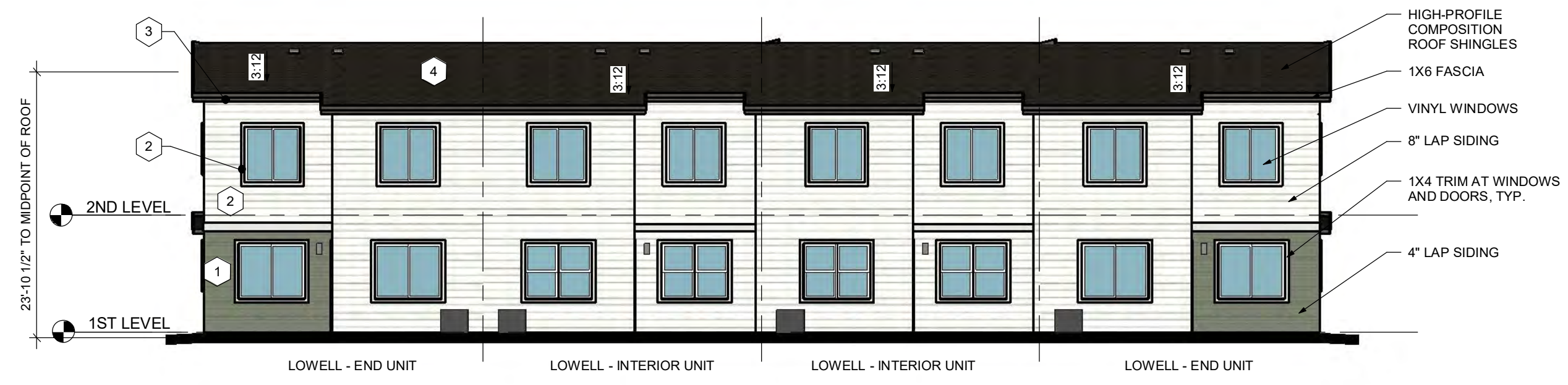
4 2-STORY FRONT LOAD - 4-PLEX - REAR ELEVATION 3/32" = 1'-0"
