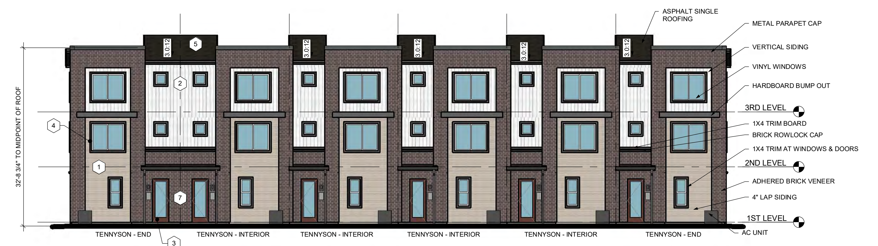
4 3-STORY REAR LOAD - 6-PLEX - FRONT ELEVATION 3/32" = 1'-0"
