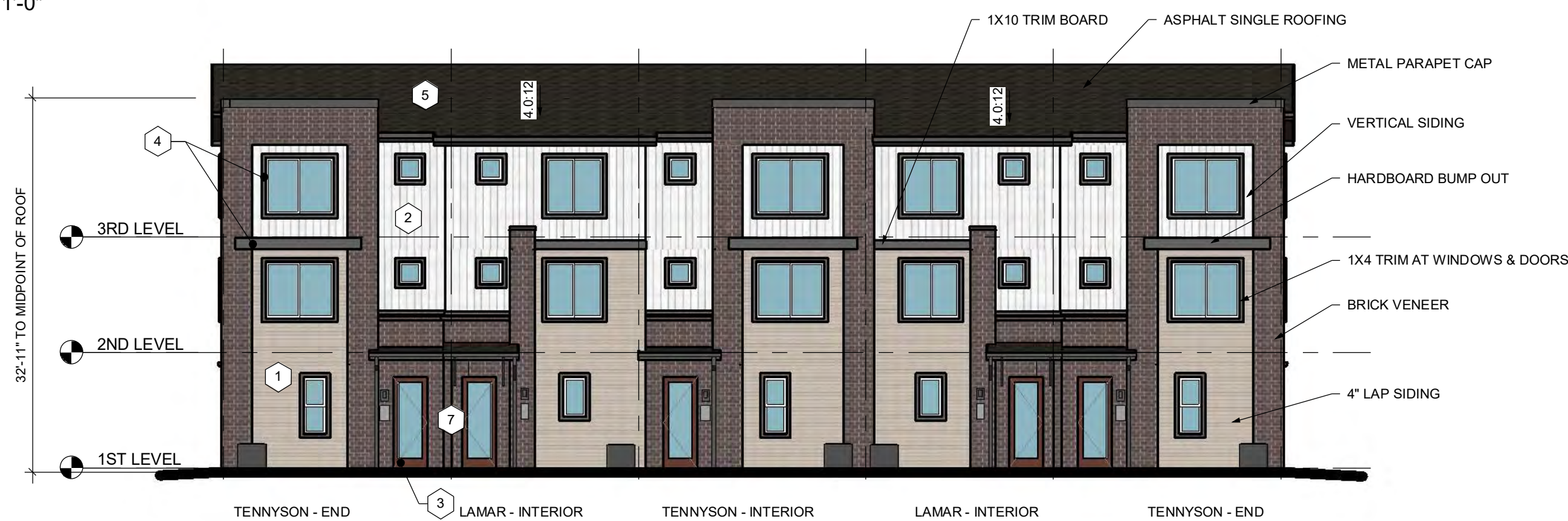
1 3-STORY REAR LOAD - 5-PLEX-B - FRONT ELEVATION 3/32" = 1'-0"
