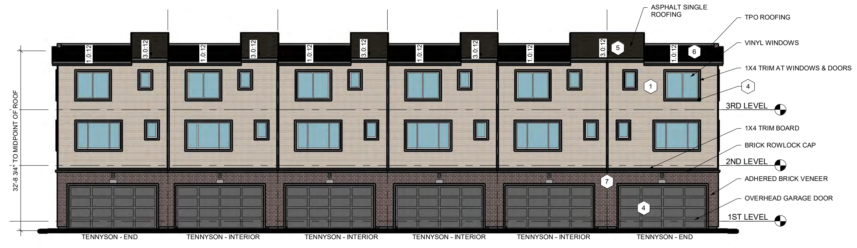
1 3-STORY REAR LOAD - 6-PLEX - REAR ELEVATION 3/32" = 1'-0"
