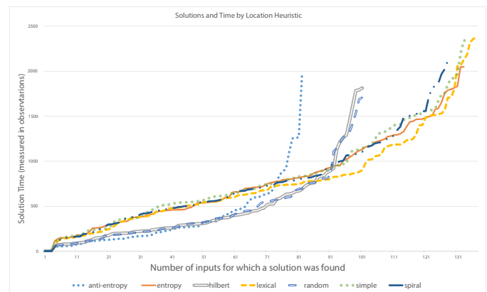
Fig. 4. Cactus plot of location (selection) heuristic experiments. Lines reaching further to the right indicate more test scenarios solved, lower lines indicate that fewer choices (observations) were required. The choice count for a solution include any restarts required because of contradictions. The default limit of 10 restarts was used. There are three clusters of performance: anti-entropy had the fewest solutions, hilbert and random had a few more, and the rest performed comparably. In general, discontinuous location heuristics tend to find solutions slightly faster but are more likely to encounter contradictions.
