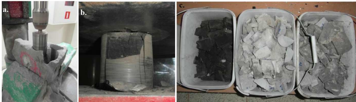
Fig. 4. Investigations into R_c of copper ores: a. sample preparation, b. shale during R_c testing, c. a scrap of shale, sandstone and dolomite after tests
