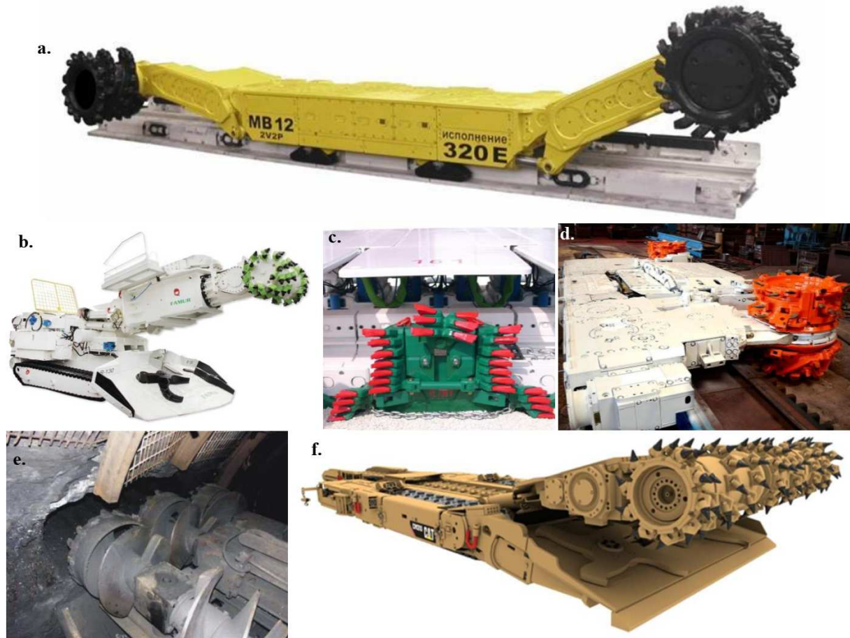
Fig. 2. Selected winning machines in underground mining: a. longwall shearer (MB12 320E TMachinery a. s.), b. roadheader (R-130 FAMUR S. A.), c. coal plough (PL 738V Ostroj a. s.), d. longwall shearer with vertical axes (KTB200 Corum Group), e. drilling shearer (VS-SEAL-625 z OKD Ostrava), f. continuous miner (CM210 CAT)
