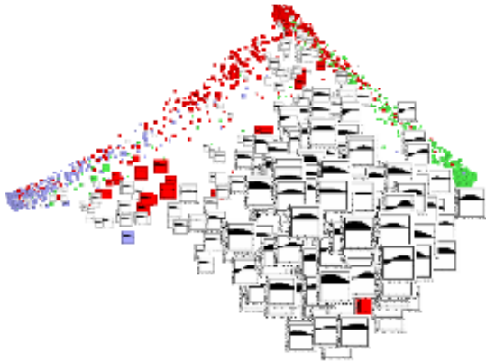
Figure 2: A close-up screenshot of a 3D glyph-supplemented scatterplot showing the performance of a linear Support Vector Machine (SVM) on a 4-way Mandarin syllable tone classification task. Ndaona embedded syllables so that those classified similarly by the SVM are close together. The glyph for each syllable represents the 20-dimensional vector input to the SVM. Syllables with the same tone are represented by glyphs of the same color; the white syllables in the foreground have falling tone.
