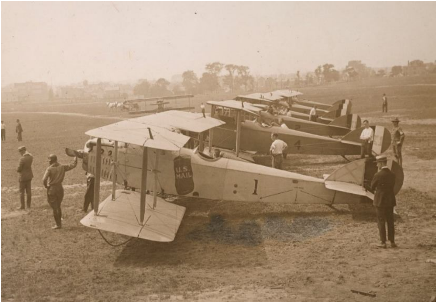
Specially-built airmail planes at Standard Aircraft Corporation in Elizabeth, New Jersey, August 1918. The Standard JR-1B mail planes had 150 HP motors and a top speed of 75 to 80 miles per hour. Strong headwinds could slow the planes down to 30 miles per hour; severe wind gusts could actually propel the planes backwards. Courtesy National Archives and Records Administration
