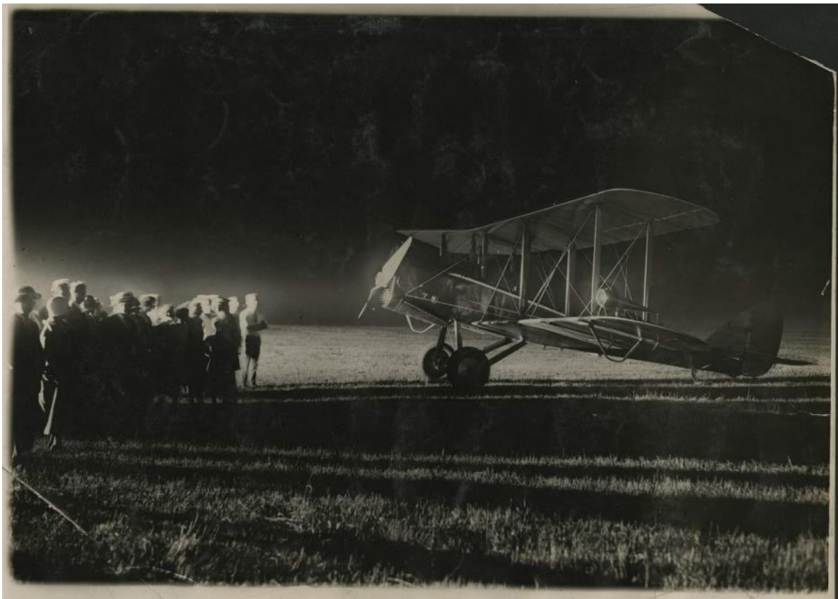
DH-4 mail plane equipped with lights on nose and wingtips, for night flying, around 1924. Courtesy National Air and Space Museum
