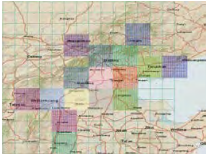
FIGURE 7.13 Example of a nested modeling system of air quality in the Jingjinji region in China
