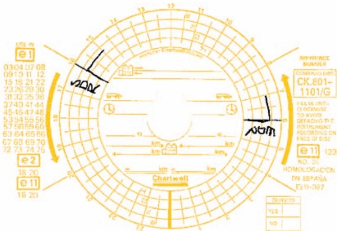
This is an example of manual entries made on the rear of a tachograph chart by a driver who started his day at 06.00 with an hour's work doing other duties away from his vehicle. He also finished his day with an hour of other work away from his vehicle and has indicated both the end and the start of a daily rest period. His activities while with the vehicle are recorded by the instrument on the other side of the chart once it has been inserted.
