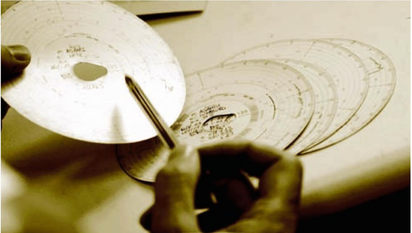
An approved tachograph is the required instrument by which the activity of drivers subject to the EU or AETR drivers' hours rules, and the vehicle's speed, distance and the time, are recorded. There are two main types of tachograph – analogue and digital.
