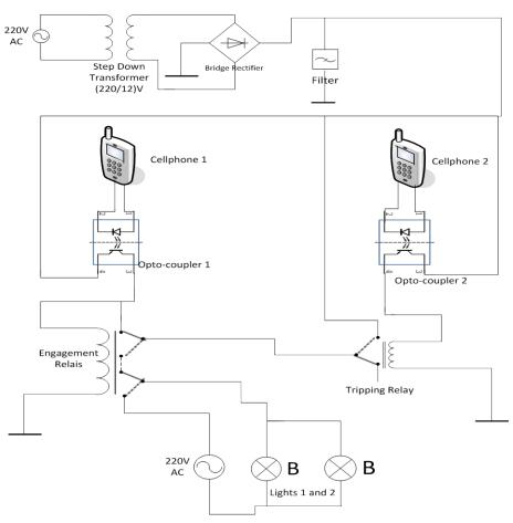
Figure 1. Design of Wireless Remote
