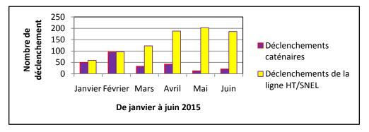
Figure 8. Statistics of tripping operations in all substations SNCC from January to June 2015
