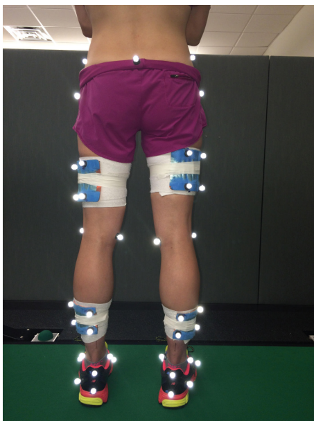
Figure 2. Retroreflective marker placement. A total of 39 markers were placed with at least 3 markers per segment were placed on the pelvis, thighs, shanks, and feet for tracking during running. Static markers were placed over the joints in order to establish anthropometrics and segment coordinate systems.
