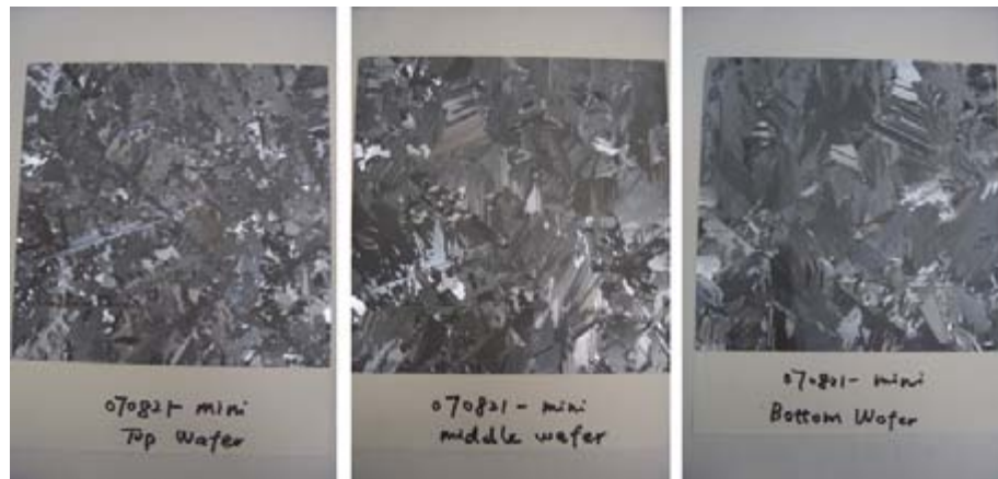
Figure 1. Pictures of wafers sliced from mini-cast ingots: 3 wafers from the top, middle and bottom locations of the doped mini-brick after KOH etching
