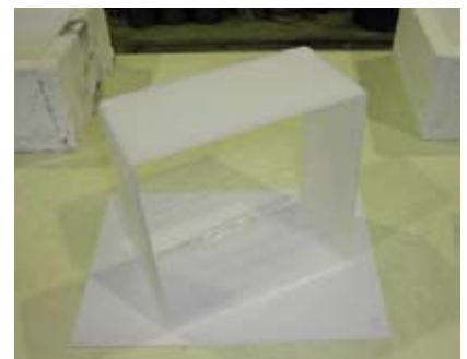
Figure 2: Photo of a 200x200x100mm 3 anisotropic quartz crucible with transparent bottom and opaque side walls.
