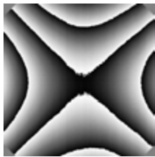
Moiré image- 140,000 data points on 156mm cell
