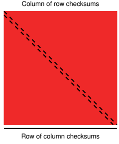
Figure 3: The encoded initial matrix
