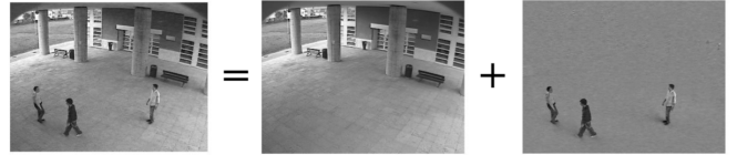
Figure 10: Sample output of Robust PCA for stationary video background subtraction
