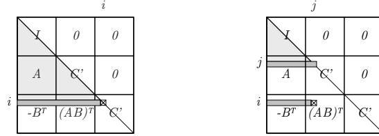
Figure 1: Dependencies of L(i, j) , for diagonal entries (left) and other entries (right). Dark grey represents the sets S_{i,i} (left) and S_{i,j} (right). Light grey represents indirect dependencies.
