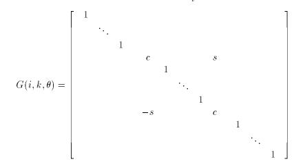
where  $c = cos(\theta)$  and  $s = sin(\theta)$  for some angle  $\theta$ . Premultiplication of a vector x by  $G(i, k, \theta)$  amounts to a clockwise rotation of  $\theta$  radians in the (i, k) coordinate plane. If  $y = G(i, k, \theta)x$ , the vector y can be described by
