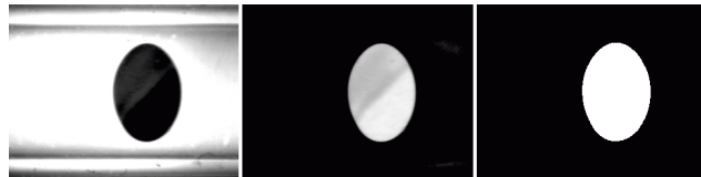
Figure 5: Image sequence depicting the segmentation procedure of a cell image scene using background subtraction.
