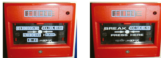
Figure 9: Detected text patches, shown by white bounding boxes, using the multi-channel classifier (left) and single channel, maximum phase congruency classifier (right).
