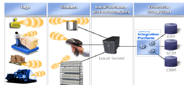
Figure 02 - Basic scheme of RFID use.
