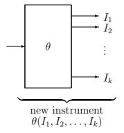
If each  $I_i$  is based on  $\mathbb{B}_{n_i}$ , the combined system is now a new instrument  $\theta(I_1, I_2, \ldots, I_k)$  based on  $\mathbb{B}_n$ ,  $n = \sum n_i$ . Of course even if each  $I_i$  is exhaustive, the new instrument may not be, since  $\theta$  may reject some copies.
