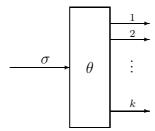
That is, a copy of a state is prepared and observed with an instrument; on the basis of the result, the copy is either rejected or is classified as belonging to one of k possible new states. We say the operation has k exits. In terms of beam physics parlance,  $\theta$  is a beam splitter, for other situations however this is merely a metaphor. In a psychological experiment for instance, the subject can be given a preliminary test, and on the basis of the result he
