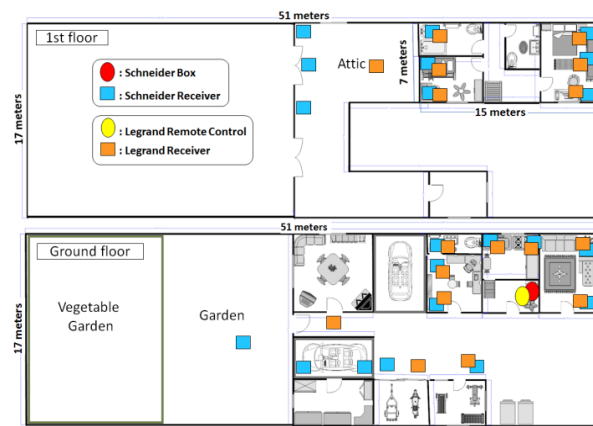
Fig. 7. ZigBee read range experimental results.
