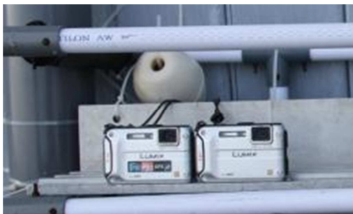
Figure 5: Low Cost Multi-View Camera Installation
