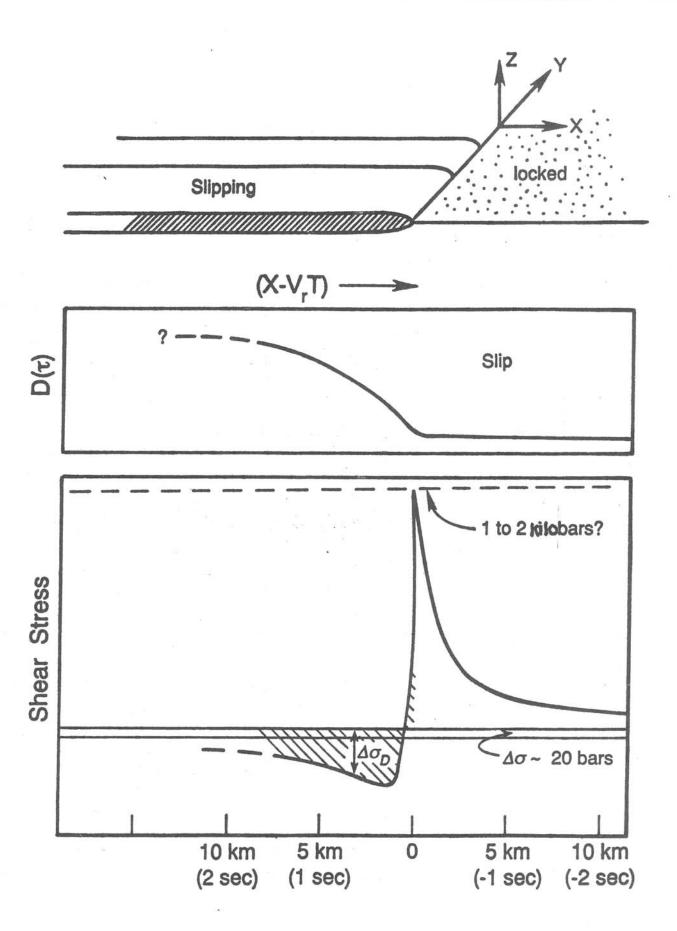
Large earthquake occurs only if rupture propagates large distances
