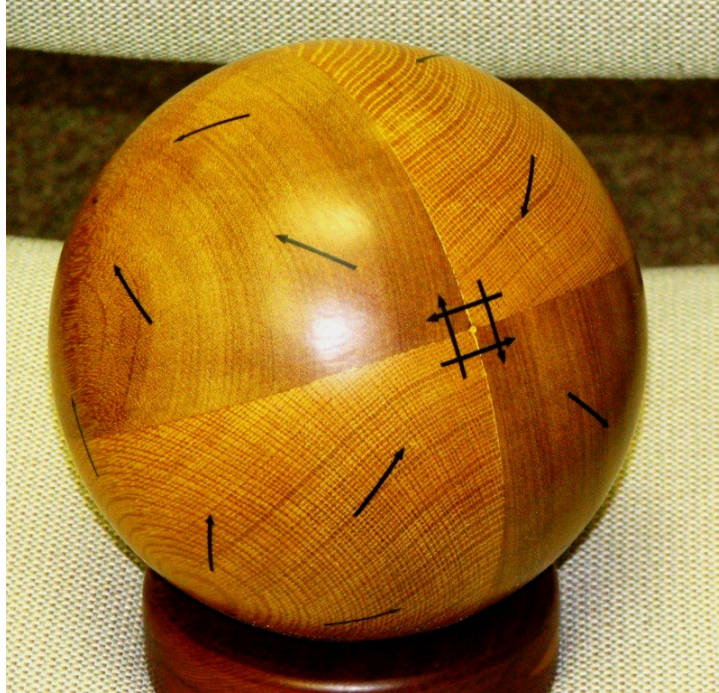
Figure 7.7. A Focal Sphere. This is an idealization of the far-field waves from a point shear at the center of the sphere. The two planes that cut the sphere are the conjugate fault planes and the sense of slip on these two planes are shown by the arrows at the intersection of the planes.
