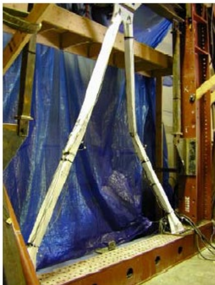
Figure 6.20 Large braces are stiff and they put large loads into a frame, but small braces can buckle in compression.
