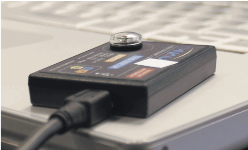
Figure 2.7 ONAVI MEMS accelerometer used by QuakeCatcher network. This is a 3-component 80 dB device with a 2 g clip level.
