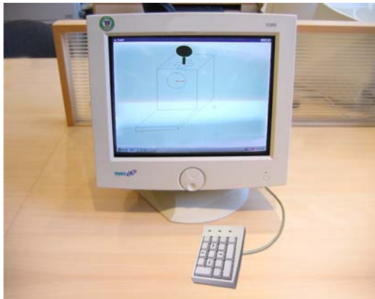
Fig. 2 The physical set up of the computer simulated lever test with a computer screen display and a control box.
