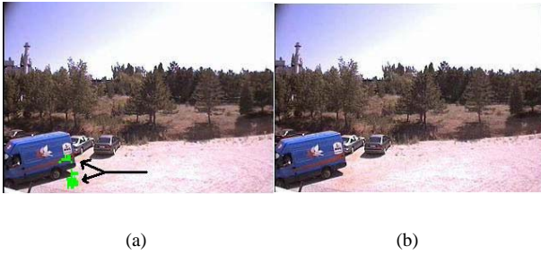
Fig. 4. (a) False alarms on the fire colored line on the moving truck and the ground with the method using color and temporal variation based method in Movie 1 in Table 1, (b) our method does not produce any false alarms.
