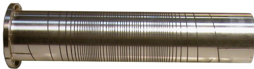
Fig. 5. Example of a solenoid of the Noack-Schweikert type
