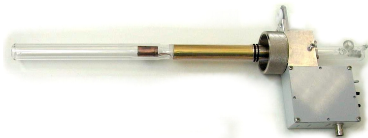
Fig. 18. A FFC signal detection probe
