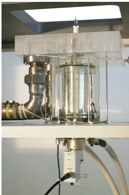
Fig. 8. The 1T magnet assembled inside its enclosure.
