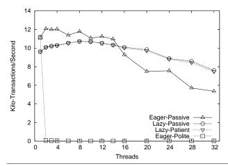
**Figure 3.** RandomGraph benchmark. The blocking "Passive" strategy avoids livelock. Polite, and other nonblocking strategies, fail to prevent livelock for eager STM with invisible reads.
