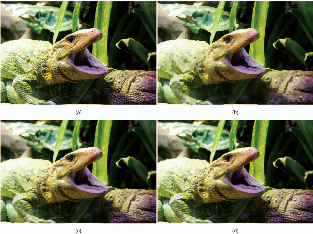
Fig. 8. Image representation using superpixels. Each superpixel from the original image (a) is colored with: (b) The average color of the original pixels in it. (c) The best linear fit to the color of the original pixels in it. (d) The best quadratic fit to the color of the original pixels in it.
