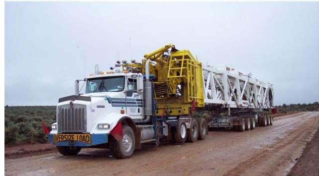
An oil derrick being hauled. Source: Colorado Motor Carriers Association
