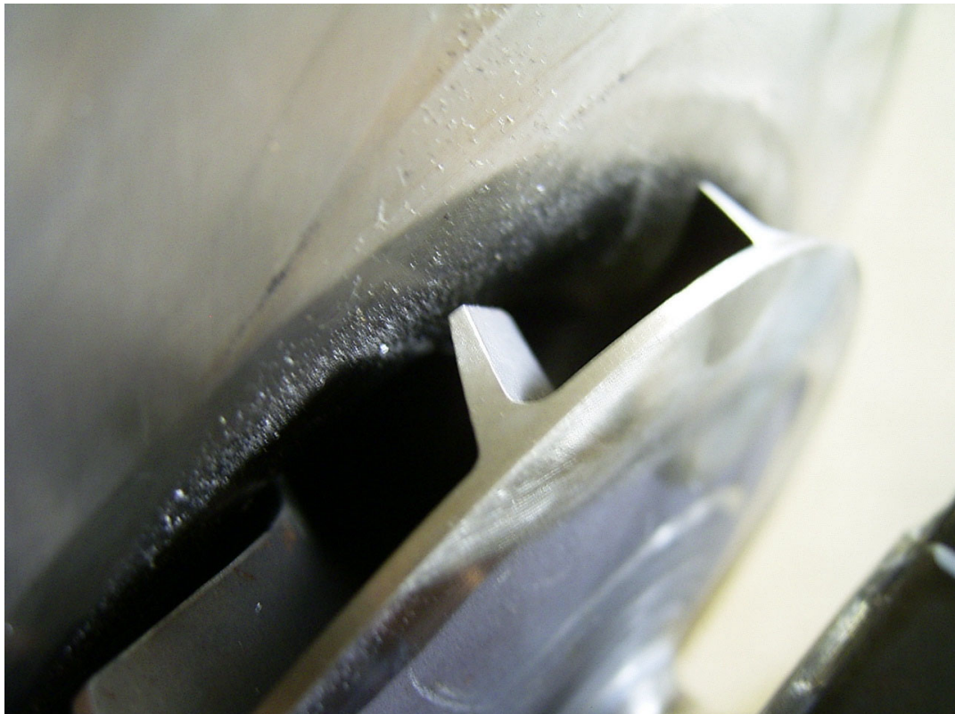
Fig 4.11 Compressor wheel trailing edges
