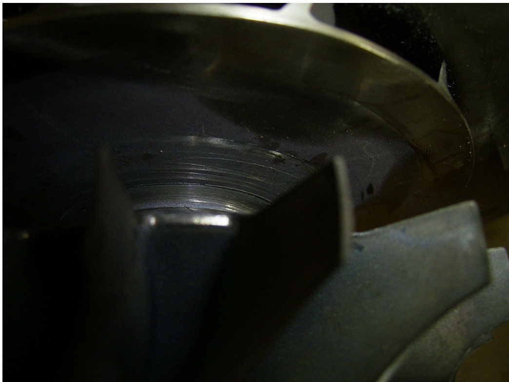
Fig 4.14 Turbine wheel leading edges
