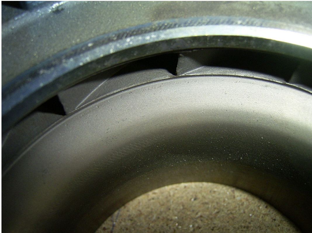
Fig 4.12 Turbine nozzle trailing edges
