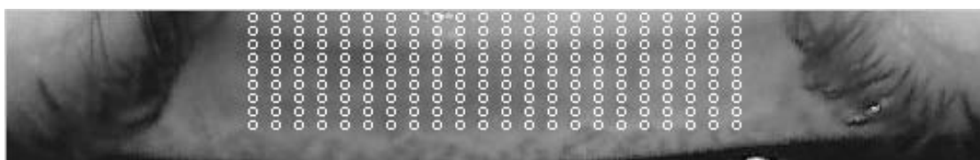
(d) Normalized iris image showing the locations at which the binary features are calculated
