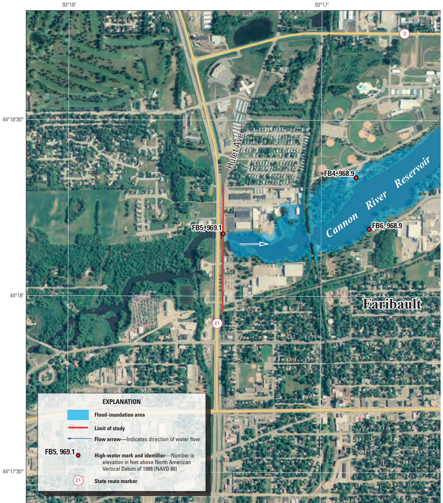
Figure 2-1. Approximate flood-peak extents and heights, flood of September 2010, for Cannon River and Straight River at Faribault, Minnesota.
