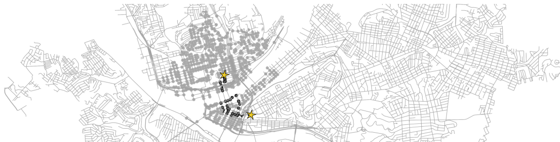
Figure 1: A standard algorithm computing the shortest path from the upper to the lower star will explore many nodes (grey), even nodes in the opposite direction. Our algorithm learns to prune to a subgraph (black) of nodes that have been included in prior shortest paths.
