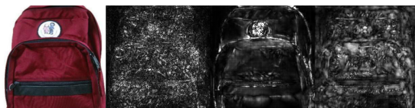
Figure 8. Sensitivity maps based on SmoothGrad (Smilkov et al., 2017) of three models. From left to right, original image, sensitivity maps of standard CNN, PGD- l_\infty AT-CNN and ST-AT-CNN.
