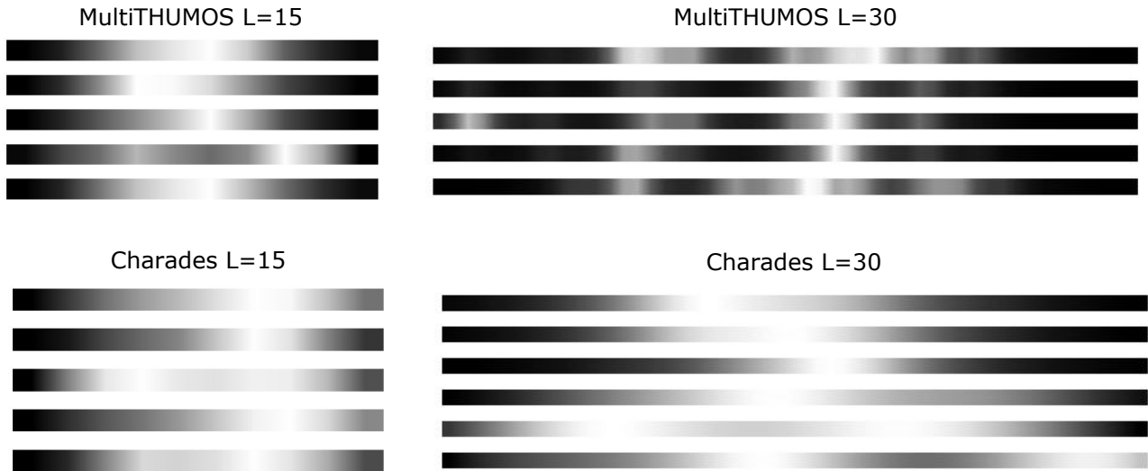
Figure 3. Illustration of several learned TGM kernels. On MultiTHUMOS, it learns to focus on shorter intervals to capture shorter events. On Charades, the Gaussians have a larger \sigma value, resulting in filters that attend to longer temporal durations.
