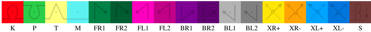
Figure 4. Top: abstract illustration and color coding of our 17 instructions. Bottom: instruction codes, which can be interpreted using the initial character of the following names: K nit and P url (front and back knit stitches), T uck, M iss, F ront, B ack, R ight, L eft, S tack. Finally, X stands for Cross where + and – are the ordering (upper and lower). Move instructions are composed of their initial knitting side ( F ront or B ack), the move direction ( L eft or R ight) and the offset (1 or 2).
