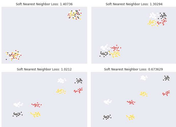
Figure 13. Data is generated for each class by sampling from two Gaussians. As entanglement is minimized using gradient descent on the (x, y) coordinates of the points, each class does not collapse into a single point; instead, both initial modes are preserved.
