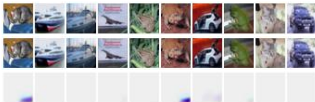
Figure 3. Original images (top) and reconstructions from i-ResNet with c = 0.9 (middle) and a standard ResNet with the same architecture (bottom), showing that the fixed point iteration does not recover the input without the Lipschitz constraint.
