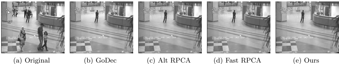
Figure 1: Background reconstruction of Hall of a business building video. (a) The original frame. (b)-(e) Background frames estimated by GoDec [58], Alt RPCA [20], Fast RPCA [56], and our algorithm respectively.
