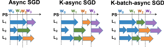
Figure 4: For K = 2 and P = 3 , we illustrate the K -async and K -batch-async algorithms in comparison with fully asynchronous SGD.
