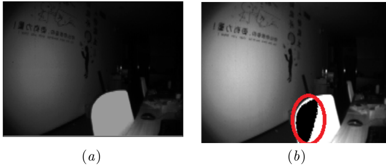
Figure 3: The intensity maps with different integration times are compared here. Firstly, it is obvious that figure (b) is brighter than figure(a). Secondly, figure(a) does not have overexposure, while figure (b) has overexposure which is circled in red. (a) No-overexposure intensity map with integration time of 400 microseconds. (b) Overexposure intensity graph with integration time of 800 microseconds, the overexposed part is the red circled part.
