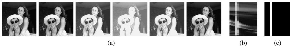
Fig. 5. Flash video detection: (a) some frames of a sequence with the flash presence; (b) visual rhythm by sub-sampling; (c) detected flash.
