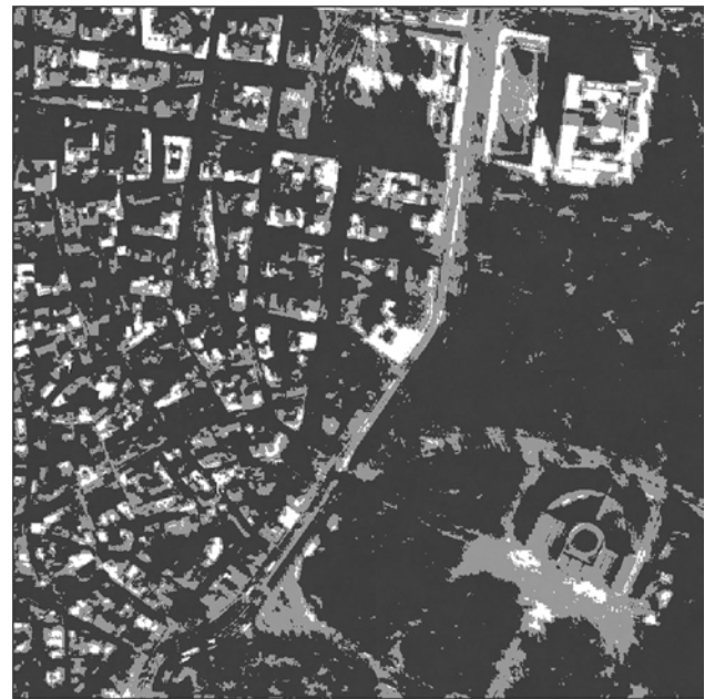
Figure 29. The unsupervised classification result of the fused image with the Multiplicative algorithm which provided the worst results.
