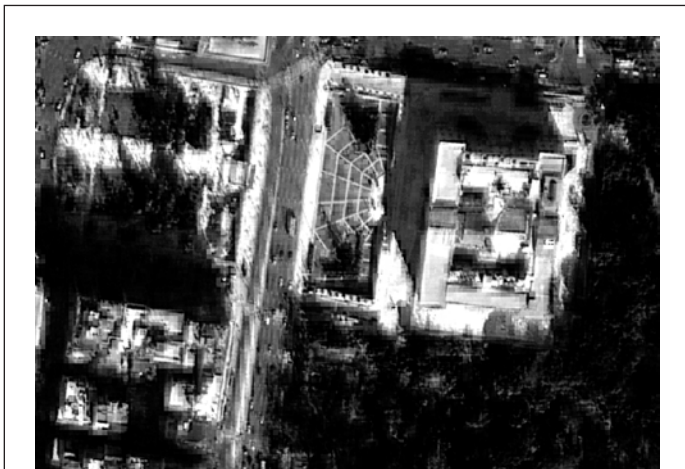
Figure 21. Distortions problems provoked by the Wavelet transform fusion technique. A color version of this figure is available at the ASPRS website: www.asprs.org .
