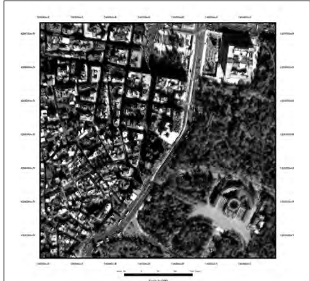
Figure 20. Fused image with the Wavelet transform (4,3,2 RGB combination). The fusion algorithm preserves the original colors exactly, but seems to present some distortions problems. A color version of this figure is available at the ASPRS website: www.asprs.org .
