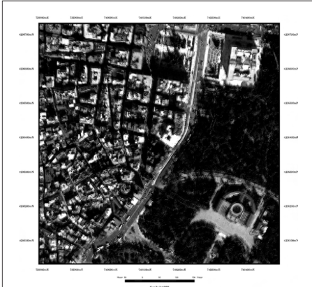
Figure 19. Fused image with the Wavelet transform (3,2,1 RGB combination). The fusion algorithm preserves the original colors exactly, but seems to present some distortions problems. A color version of this figure is available at the ASPRS website: www.asprs.org .
