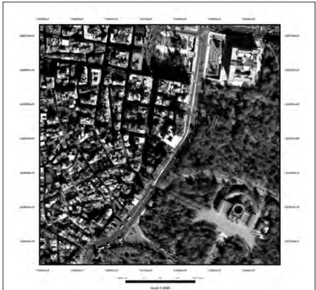
Figure 14. Fused image with the modified IHS transform (4,3,2 RGB combination). The algorithm preserves the colors of the original image. A color version of this figure is available at the ASPRS website: www.asprs.org .
