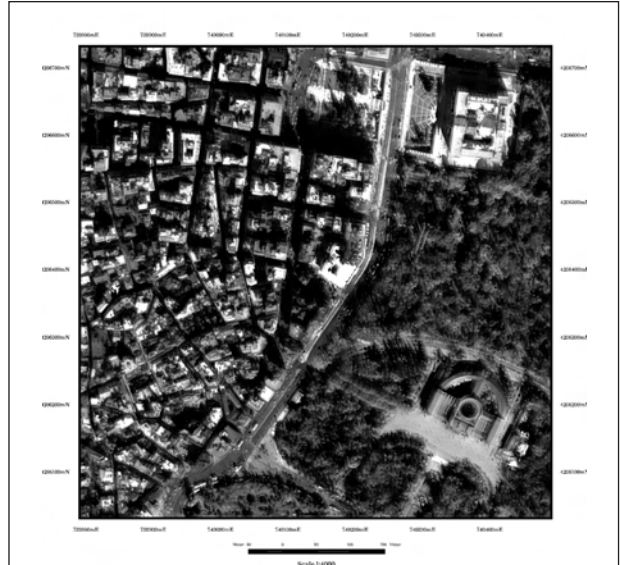
Figure 12. Fused image with the LMVM transform (4,3,2 RGB combination). The trees and the cars can be easily distinguished. The colors of the original image remain invariable. A color version of this figure is available at the ASPRS website: www.asprs.org .
