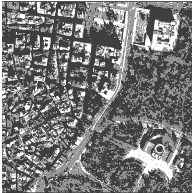
Figure 30. The unsupervised classification result of the fused image with the Pansharp algorithm which provided the best results.
