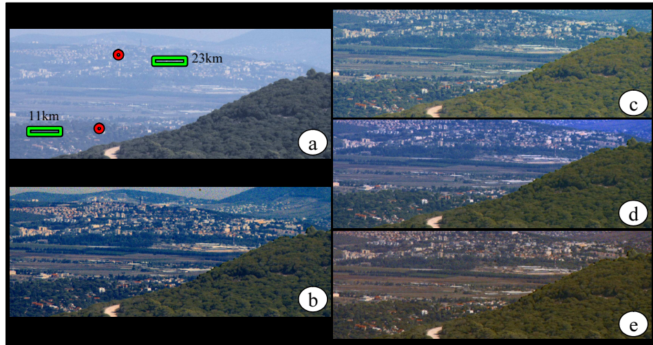
Fig. 1. Dehazing of Scene 1 (distant up to 34 km). (a) The best polarized image. The two circles mark buildings. The rectangles mark arbitrary points at different distances. (b) The environmental parameters are estimated using the sky (sky-based dehazing). (c) Result of a feature-based method assisted by ICA (d) Result of a distance-based method assisted by ICA (e) Distance-based result.
